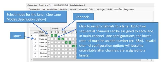
Figure 6. Channel to Lane Mapping
