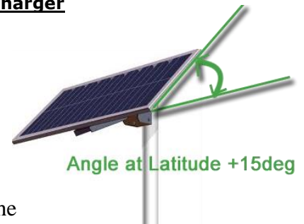
Recommended Solar Panel Angle
