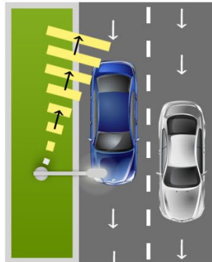
Armadillo on the side with 2 lanes incoming. No outgoing lanes can be detected
