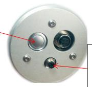
IP67 Rated M8 Connector for 12V nominal solar panel or provided external +24VDC charger.
