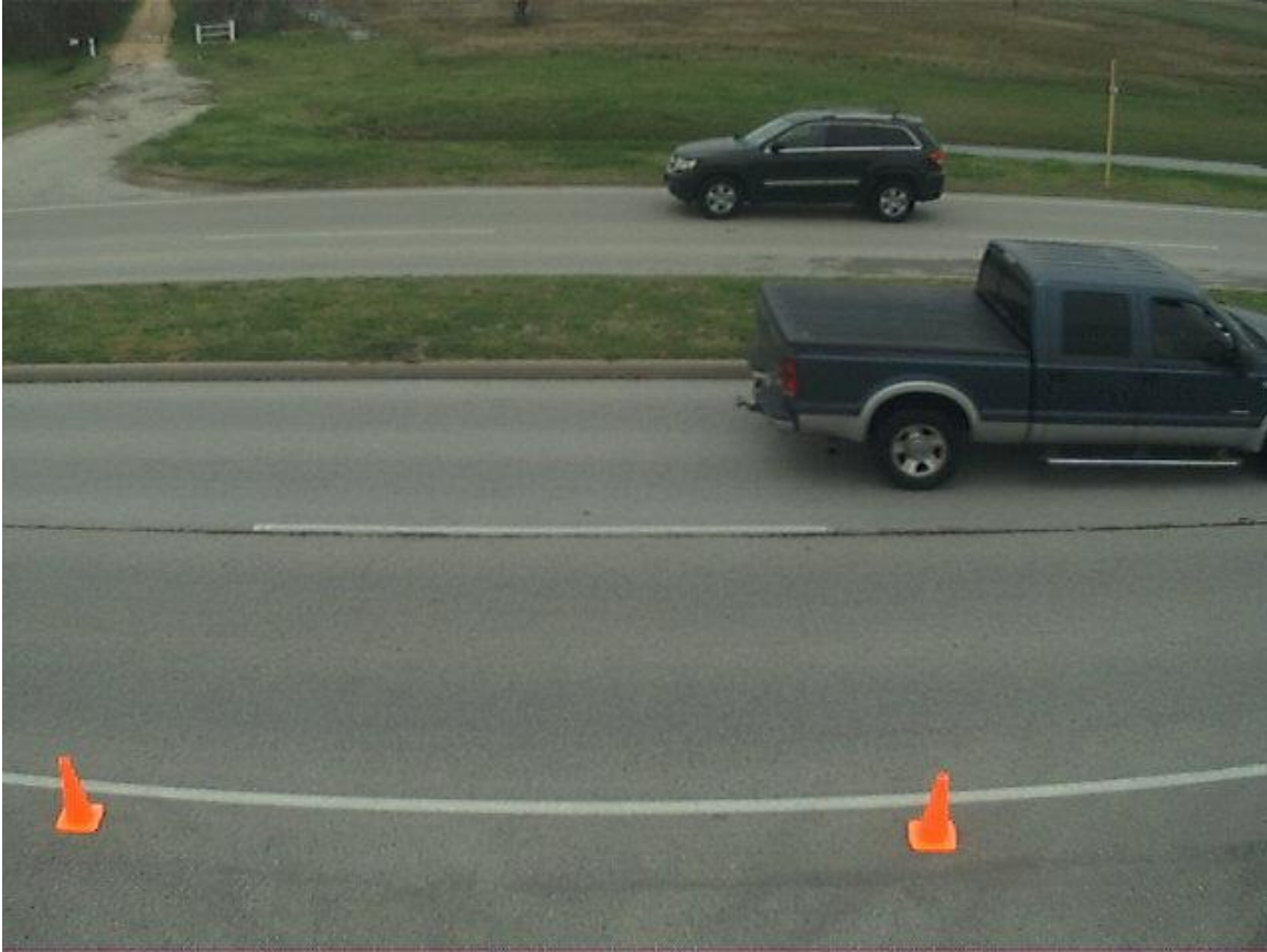
An example photo from the Armadillo Crossfire sighting camera showing proper pointing for a 4 lane highway.
